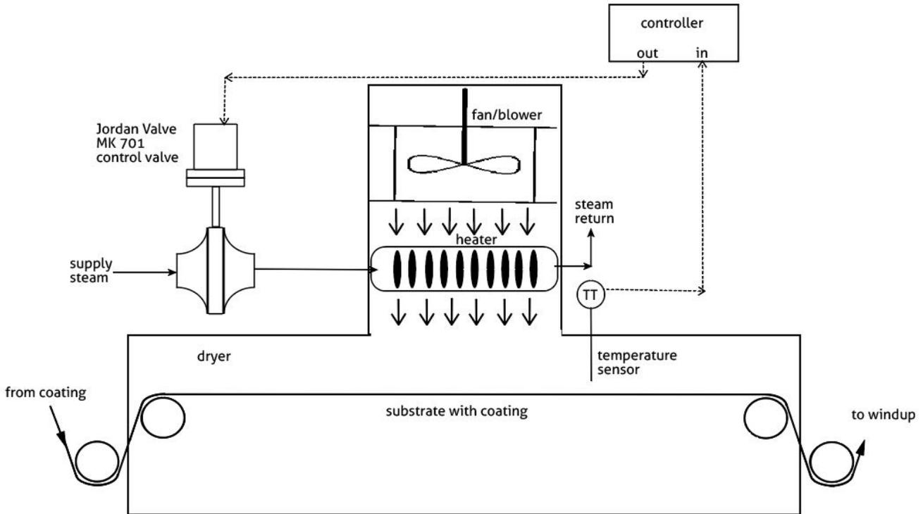
*Schematic of a coating process using Jordan MK 701 to control steam supply to the dryer*
