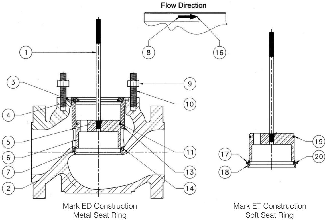
Figure 5: Body Assemblies, Mark E Series 8" Globe Valves
