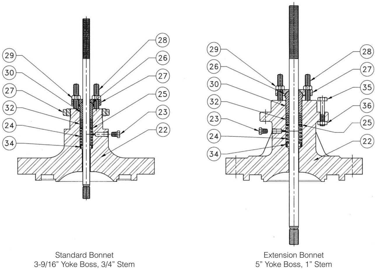
**Figure 4: Bonnet Assemblies, Mark E Series 8" Globe Valves**
