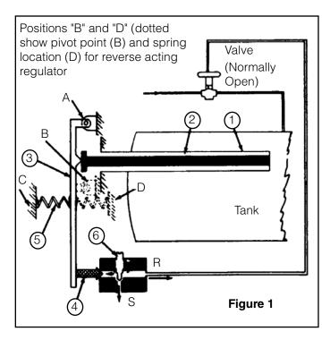
A temperature change in the medium being controlled creates a change in length of the sensitive tube (1). An increase in temperature lengthens the sensitive tube (1) and moves the Invar rod (2) away from the lever (3). The lever (3), which pivots at Point A, moves to close the exhaust valve (4) by the spring (5). This permits the supply (air or water) (S) to increase the pressure in the control line (R) and close the normally-open valve.
