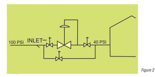
Increasing or decreasing the amount of force applied to the spring establishes the set point for a self-contained regulator.
