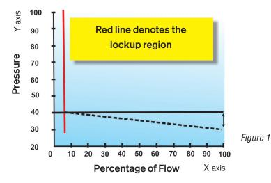
Droop is an inherent characteristic of all self-operated and pilot-operated regulators.
