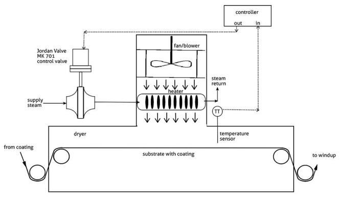
Schematic of a coating process using Jordan MK 701 to control steam supply to the dryer
